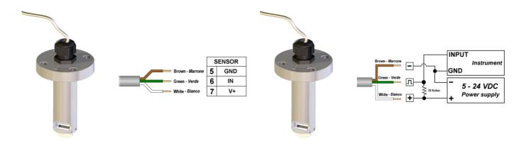
• A 2.7 KOhm Pull-up resistor may be necessary
